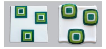
Above: a single-thick square of glass with smaller square stacks placed *unevenly*, then Full Fused. The perimeter of the piece becomes distorted because of the uneven distribution of glass. (Note that both of these tiles were created for demonstration purposes only. Incorporating wide variations of thin and thick areas in a Full Fused design can often result in breakage!)
