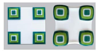
Above: a single-thick square of glass with smaller square stacks in each corner. After Full Fusing, the thin areas draw in; the thicker areas push out as the uneven layers seek equilibrium.
